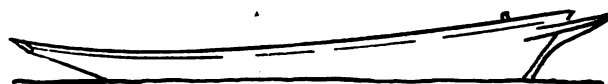
The upcurve aft that the parabolic curve gave prevented the overhang from looking drooped, and made them appear light and graceful.
